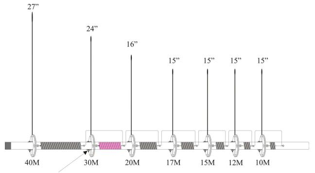
You may loosen the radial ring mounts to make it easier to align the ring holes when inserting the rods. Tighten them back when all four rods are in.
