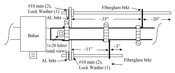
Figure 4: 6 and 2-meter stub assembly and mounting
