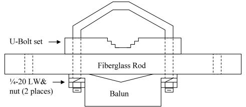
Figure 2: Balun/Center Insulator Assembly – Top View
